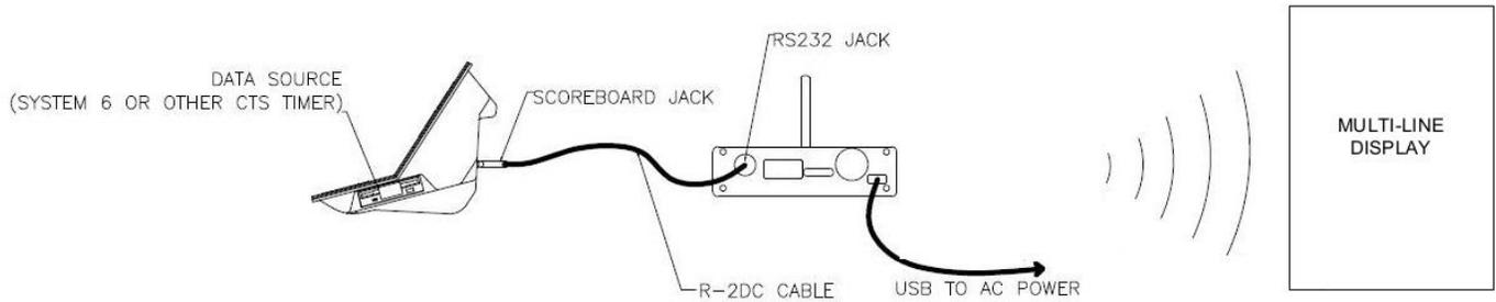
**When using a wireless connection, the WA-2 wireless adapter and scoreboard must be set to the same channel and PAN. Follow the WA-2 user instructions to change its channel and PAN. Follow instructions on previous pages if scoreboard Channel and PAN must be changed.**
