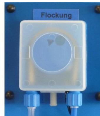
Figure 13, Flocculant dosing pump
