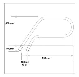
The AQUEAS AQ-GR08 P style can be used in applications when niche steps are used with pool grates.
