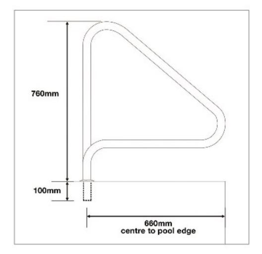
The AQUEAS AQ-GR06 in-line Grab Rail which is suited for residential applications. This can be used for commercial applications as well.
